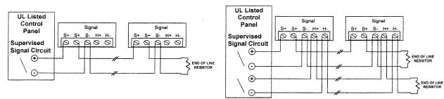
CAUTION: When using only a single power source to energize the strobe and horn (switches 1 and 2 up), the in/out wiring must be under the S+ and S- terminals only. Failure to do so may result in damage to your signal. For the horn only (GEH24) and strobe only (WGES), only the top three terminals are to be used.
