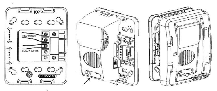
CAUTION: A jumper card is provided to test for correct wiring in the supervisory mode only. DO NOT pass alarm current through the jumper.
